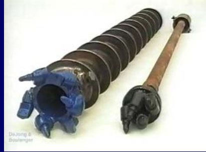
HSA outer and inner assembly with stepwise center bit
